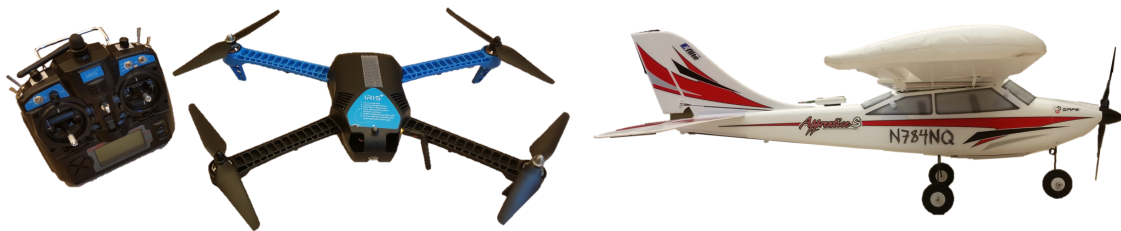
(a) Iris+ 3D Robotics quadrotor with transmitter (b) Apprentice S15e fixed-wing aircraft
