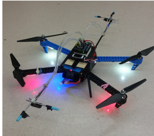
Figure 28. Quadrotor FMS vibration testing
