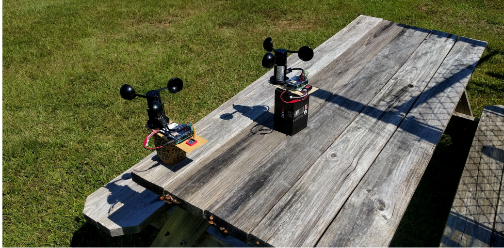
Figure 56. Anemometer validation ground test
